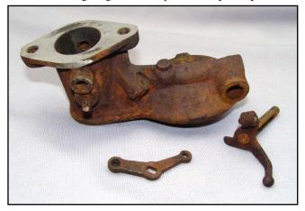
opened in my garage until last night when I tackled a really rusty carburetor. I have an ultrasonic cleaner that I put all my carburetor parts in (including the castings). The solution cuts all the oils and greases from the parts - but it doesn't remove rust. I cleaned all the parts in the ultrasonic and then submerged a very rusty carburetor casting, a choke lever arm, and some rusty bolts in the Evapo-rust. I stirred the brew with my finger and it didn't fall off.
