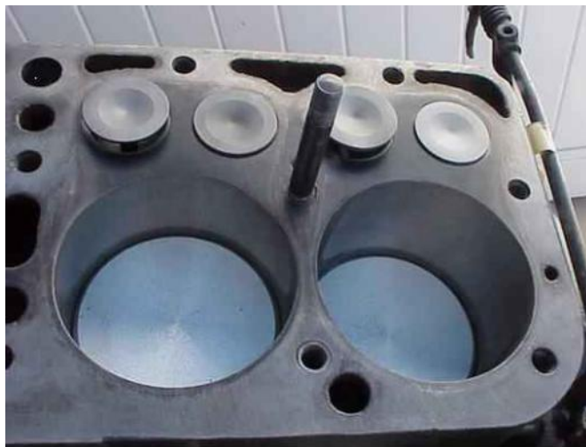
The area between #3 and #4 cylinder is a common place for a blown head gasket. The #8 stud sits right next to the area.
