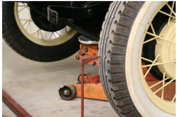
FORD SERVICE BULLETIN September 1928, page 283 fig. 576: Front wheel toe-in should be \frac{1}{16} of inch, plus or minus \frac{1}{32} (A greater than B).
