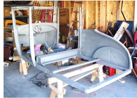
Fitting repaired quarter panels.
