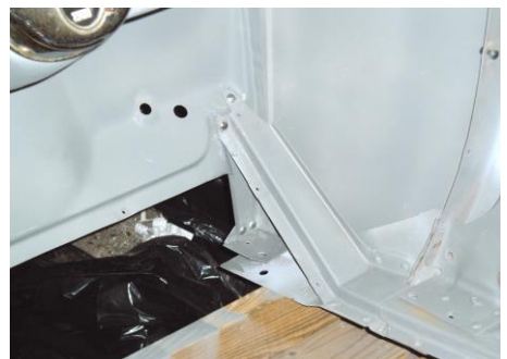
Riveting floorboard risers to firewall after welding and repairs.
