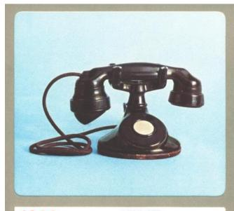
1928 America got a new look in telephones in 1927 when the combined receiver and transmitter idea, used since 1878 by telephone linesmen, was sufficiently improved to be adapted for general service. It was popularly known as the "French phone" because it resembled continental instruments.
