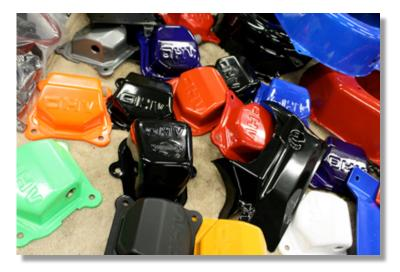
Because the powder coating must be baked, typical body fillers cannot be used. There may be some metal type fillers available that can withstand the baking temperatures. Existing powder coats can be coated over but adhesion is dependent on the original coat. Clear coats can be applied but the clear can change the color slightly. Jimmy has powder coated a variety of items including lawn furniture and Yeti cups. Coatings can be applied as a two-tone but the process is more tedious.
