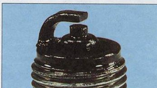
Oil fouling – Wet oily deposits leading to misfire and weak spark. Caused by oil leakage past piston rings or valve guides (4-stroke engine), or excess lubricant (2-stroke engine).
