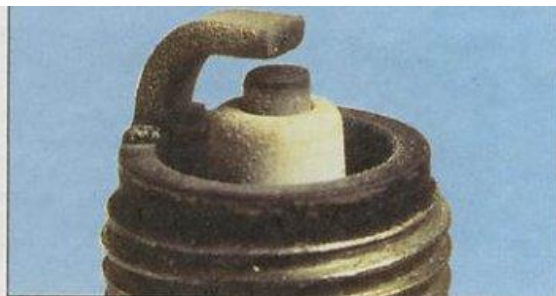
Normal condition – A brown, tan or grey firing end indicates that the engine is in good condition and that the plug type is correct.
