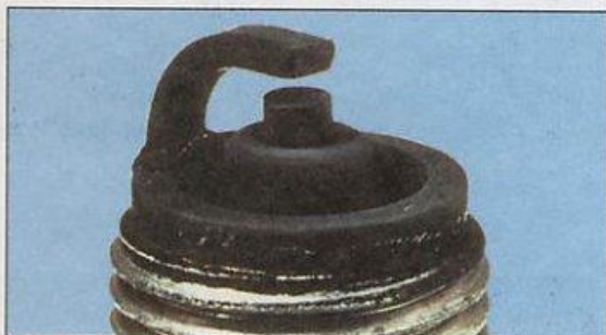
Carbon fouling – Dry, black sooty deposits leading to misfire and weak spark. Caused by an over-rich fuel/air mixture, faulty choke operation or blocked air filter.
