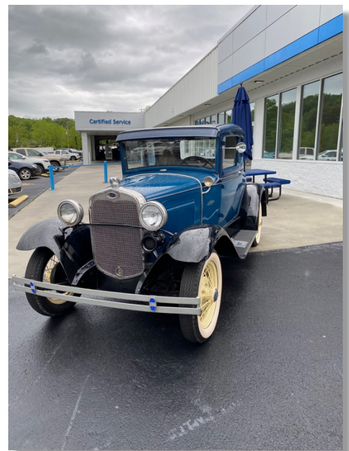
Found at Countryside Chevrolet in Franklin, North Carolina: 1931 Model A coupe with indented firewall but with 2-piece splash aprons and 1930 radiator shell. Photo by Matt Barrett
