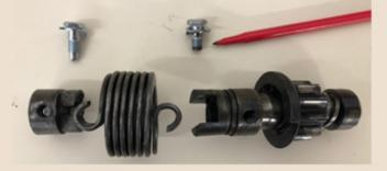
The other bolt is "special" only because it is only 11/16" long. This allows the bolt to lock the spring in place, without having the bolt actually touch the starter shaft. Don't be tempted to use a 3/4" long bolt instead of the correct shorter one. See the comparison photo of a 3/4" bolt and the correct bolt.
