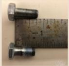
When this longer bolt is used, it presses against the starter shaft when tight and it messes up the Bendix operation.
