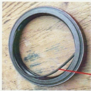
The rear main seal has a garter spring that is to be removed.
