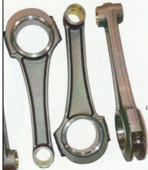
Forged steel connecting rods swing with clearance and strength.
