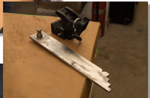
John Buchanan's brake adjusting tool that uses a motorcycle frame clamp to hold the tool to the steering column.
