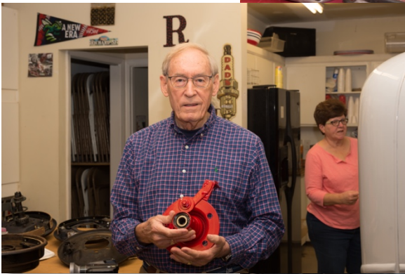
Stuart Smith with his brake centering tool fabricated from a front wheel hub.
