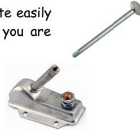
So you want to make the rod a bit harder to turn when installing it in the switch. Add a small drop of blue thread locker to the rod before you screw it in, or gently tap the threads a little with a hammer to deform them and make them harder to screw in and out.
