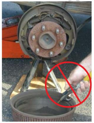
Using compressed air, a brush (wet or dry), or a dry rag to clean brake assemblages has the potential to expose you to asbestos fibers.
