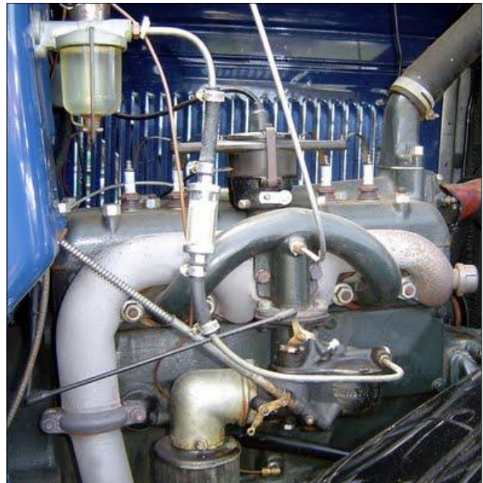
Figure 1: Model A Carburetor Arrangement
